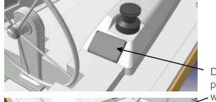
Dedicated instrument positions for tiller and wheel steering option, incl 7" plotter
