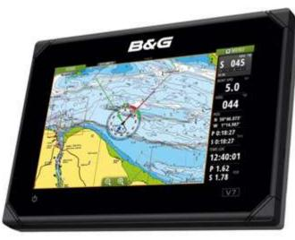
B&G V7 integrates with your on board instruments to unlock awardwinning sailing features including SailSteer<sup>™</sup> and Sailing Time to view crucial sailing data all on one screen or alternatively overlaid on your chart. With built in Wi-Fi, Triton display, with unrivalled 170° viewing angles, a large 4.1-inch display, an optically bonded glass screen for zero condensation and a menu system that is as easy to use as it is practical.
