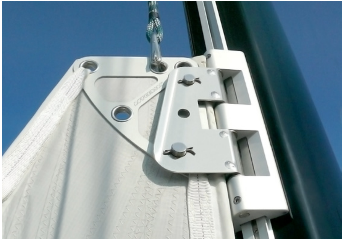
3 Car slide system with masttrack for easy mainsail hoisting.
