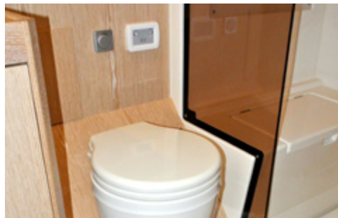
Electric toilet with sea water flush
