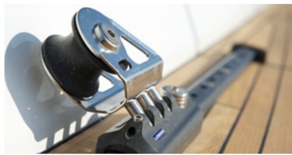
Extra track with pin stop cars for larger 105% genoa
